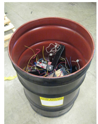
A 30 gallon drum of lamp ballasts
